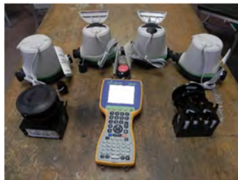
Commonly Used Radio Read Water Meters
